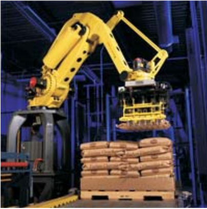
PALLETIZING CEMENT BAGS
